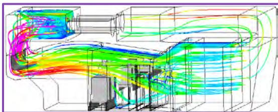
stimulants development, and Computational Fluid Dynamics (CFD) modeling analysis for the design of the aerosol circulation chamber. This multi-year program required extensive coordinating of scientific and engineering resource to achieve a successful fabrication and implementation of the WSLAT project.
